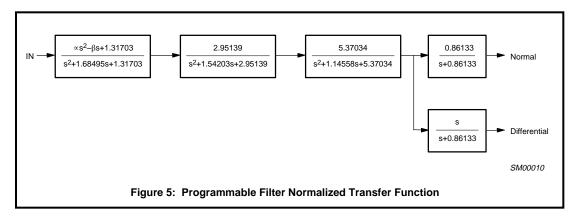
With a zero at the origin, the filter provides a time-differentiated filter output. This is used in time qualification of the peak detection. To ease the timing requirement in peak detection of a signal slightly above the qualification threshold, the time-differentiated output is purposely delayed by 1.2 ns relative to the normal low pass output.
